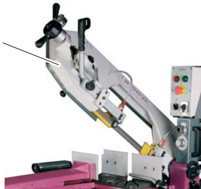
Img. 1-3: Saw belt housing with protective cover.
