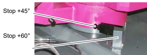
Img.4-8: Angle cut from 0° to +60°
