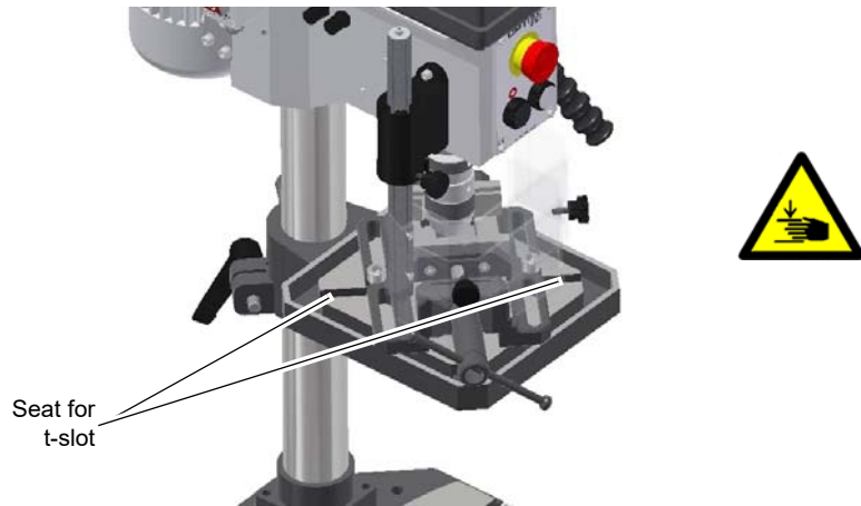
Img. 1-2: Drilling table
