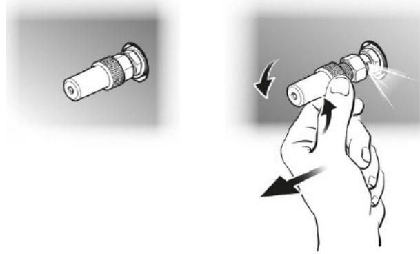
Fig. 9: Safety valve with ring nut
