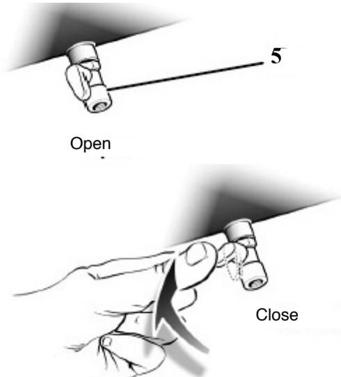
Fig 8: Drain valve
