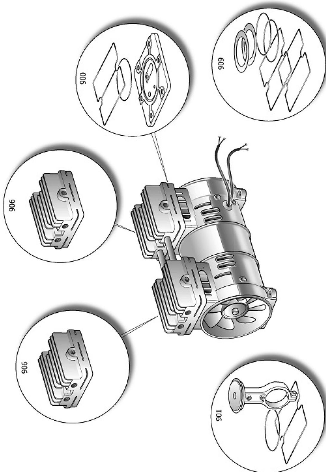
Fig. 11: Spare parts of pump assembly
